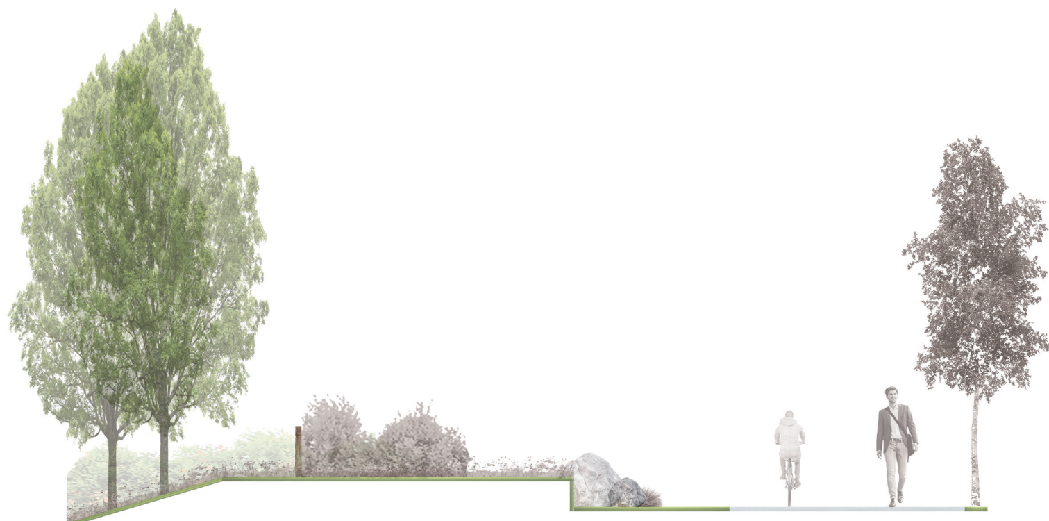
Fig.23 - Section showing cycle path and boulders retaining slope and new native hedgerow.
